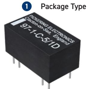
The Series 97 is a range of reed relays with pins in the popular Dual-in-Line format.
