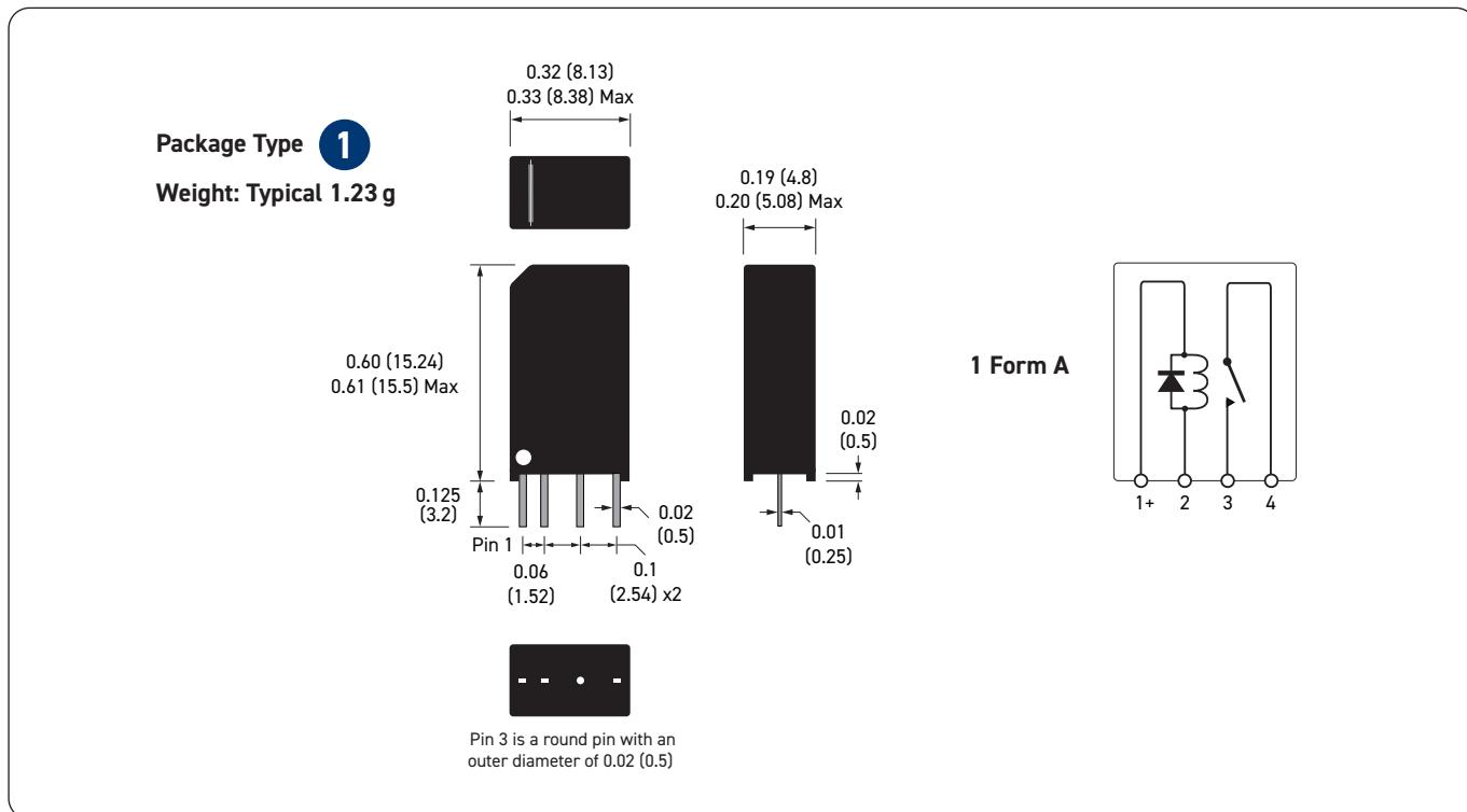
**Important:** Where the optional internal diode is fitted the correct coil polarity must be observed, as shown by the + symbol on the schematics. Pin 1 is the positive connection.
